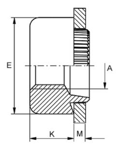
Female thread A = M6Height K = 5.0Outer diameter E = 10.0Plate thickness = 3.2 to 3.4
